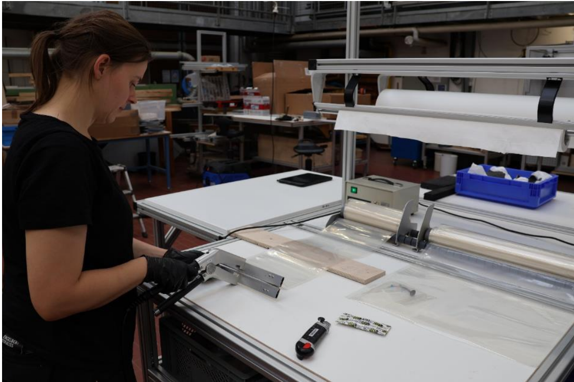
Workplace for sealing metal objects in gas-barrier bags @Inga Vollmer-Bardelli, LEIZA
