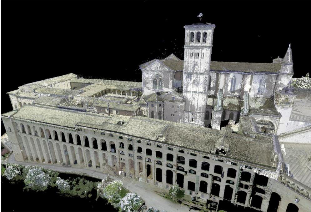
*Fig. 9 Sacro Convento of Assisi: 3D point cloud perspective © Vigili del Fuoco*
